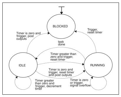
Figure 8-7. New STD for ATR Triggered Tasks
